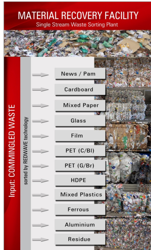
Infeed material is sorted in 12 different fractions
